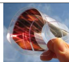
Power supply (organic photovoltaics, flexible battery, ...)
